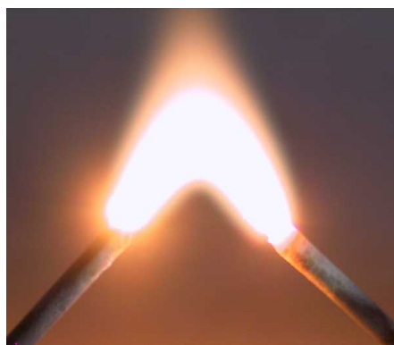
Figure 11. Example of Arc Flash Between Two Conductors (Grochowski, 2008)
